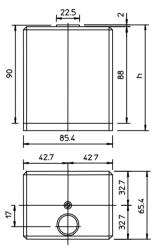
h: Dimensions depending on the type of socket: 95 with socket A 99 with socket B 98.3 with socket N
