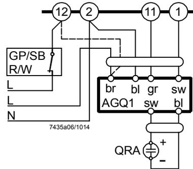
Burner with fan control via auxiliary contactor (HS) with air pressure switch (LP)
