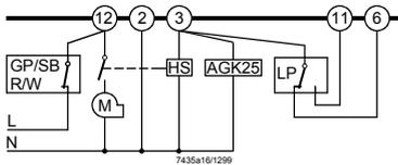
QRA with auxiliary unit AGQ1.xA27 with LGB21 (diagram 7435a06)
