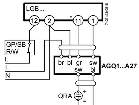
Measurement made on the flame detector
