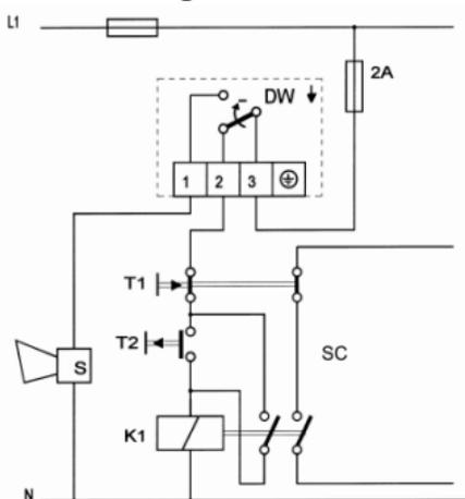
Fig. 6. Limitation de pression minimum
